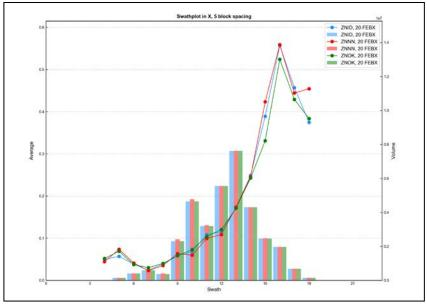
Figure E - 46 Swath Plot in the X Direction of Total Zinc for the Iron Oxide Breccia
