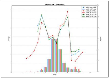
Figure E - 73 Swath Plot in the X Direction of Silver for the Magnetite Skarn
