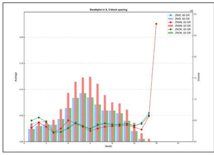
Figure E - 106 Swath Plot in the X Direction of Total Zinc for the Granite
