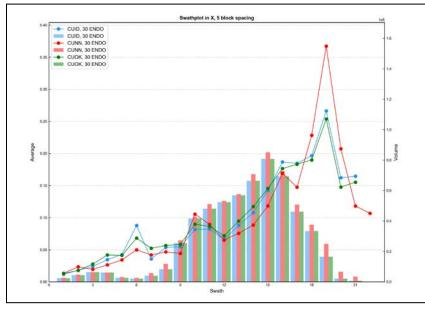
Figure E - 55 Swath Plot in the X Direction of Total Copper for the Garnet Skarn
