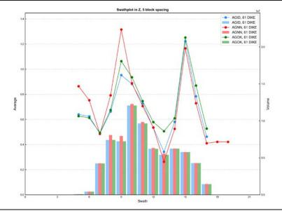
Figure E - 111 Swath Plot in the Z Direction of Silver for the Dikes
