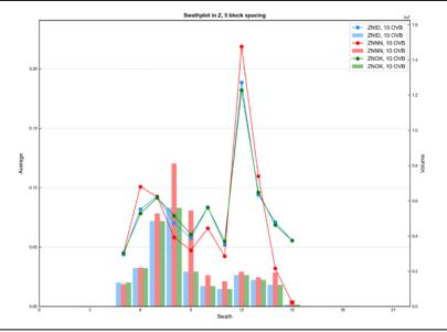
Figure E - 24 Swath Plot in the Z Direction of Total Zinc for the Overburden
