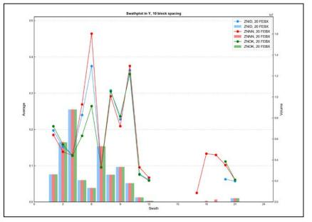
Figure E - 47 Swath Plot in the Y Direction of Total Zinc for the Iron Oxide Breccia
