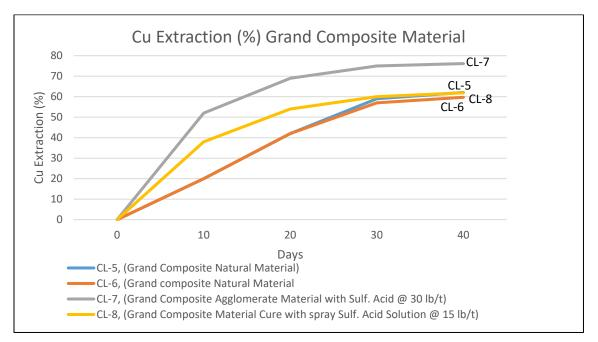
Figure 13-3 Copper Extraction - Grand Composite Column Tests
