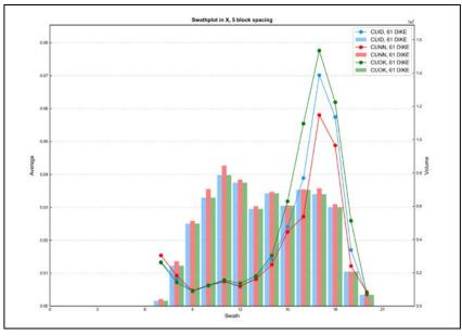
Figure E - 115 Swath Plot in the X Direction of Total Copper for the Dikes
