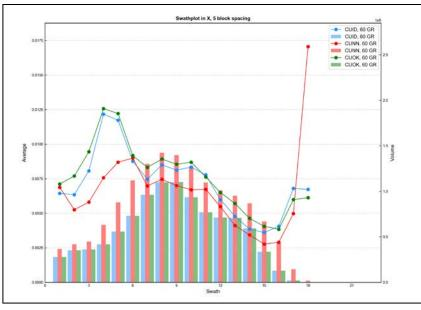
Figure E - 103 Swath Plot in the X Direction of Total Copper for the Granite
