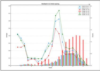
Figure E - 91 Swath Plot in the X Direction of Total Copper for the Limestone
