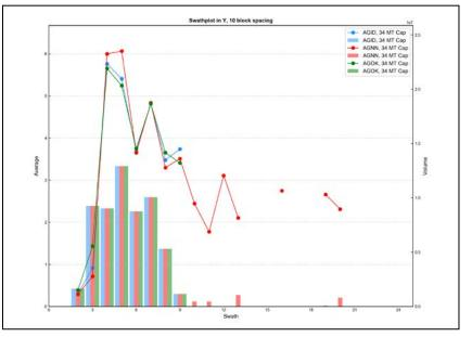
Figure E - 74 Swath Plot in the Y Direction of Silver for the Magnetite Skarn
