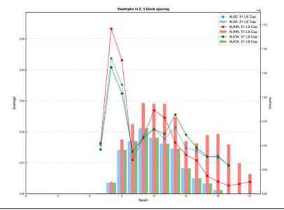
Figure E - 90 Swath Plot in the Z Direction of Gold for the Limestone
