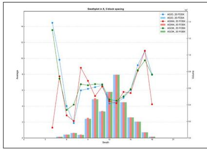
Figure E - 37 Swath Plot in the X Direction of Silver for the Iron Oxide Breccia
