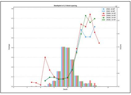
Figure E - 82 Swath Plot in the X Direction of Total Zinc for the Magnetite Skarn
