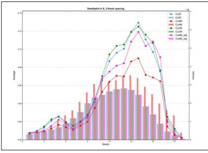
Figure E - 7 Swath Plot in the X Direction of Total Copper for the Global Resource
