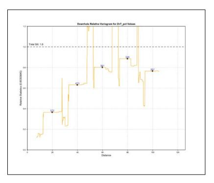
Figure D - 172 Downhole Variogram for Total Zinc in Granite
