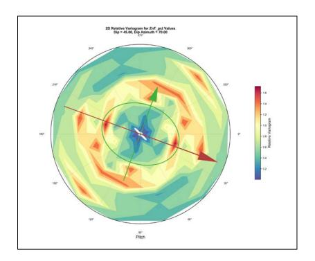
Figure D - 171 Radial Plot for Total Zinc in Granite
