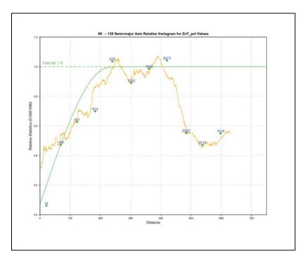
Figure D - 164 Semi-Major Axis Variogram for Total Zinc in Magnetite Skarn
