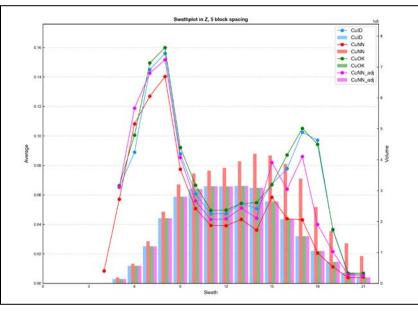
Figure E - 9 Swath Plot in the Z Direction of Total Copper for the Global Resource
