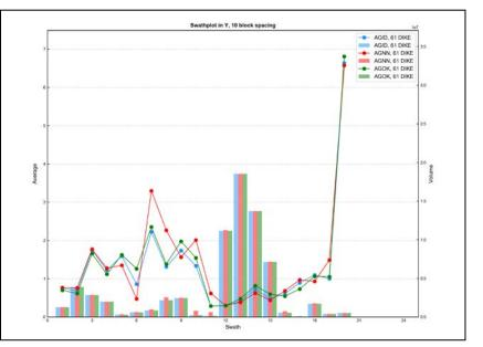
Figure E - 110 Swath Plot in the Y Direction of Silver for the Dikes
