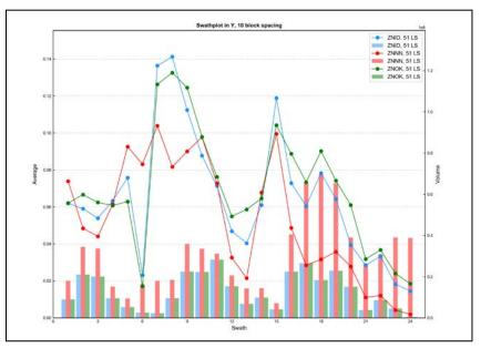
Figure E - 95 Swath Plot in the Y Direction of Total Zinc for the Limestone
