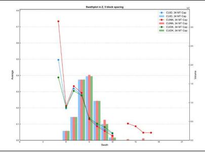
Figure E - 80 Swath Plot in the Z Direction of Total Copper for the Magnetite Skarn
