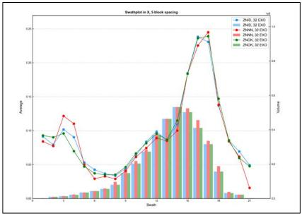
Figure E - 70 Swath Plot in the X Direction of Total Zinc for the Pyroxene Skarn
