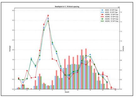
Figure E - 26 Swath Plot in the Y Direction of Silver for the Granite Porphyry
