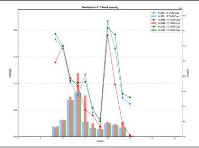
Figure E - 18 Swath Plot in the Z Direction of Gold for the Overburden
