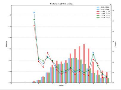
Figure E - 33 Swath Plot in the Z Direction of Total Copper for the Granite Porphyry
