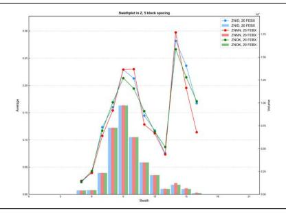
Figure E - 48 Swath Plot in the Z Direction of Total Zinc for the Iron Oxide Breccia
