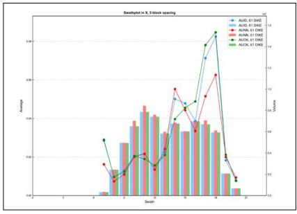
Figure E - 112 Swath Plot in the X Direction of Gold for the Dikes
