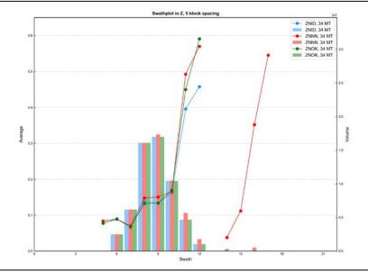
Figure E - 84 Swath Plot in the Z Direction of Total Zinc for the Magnetite Skarn
