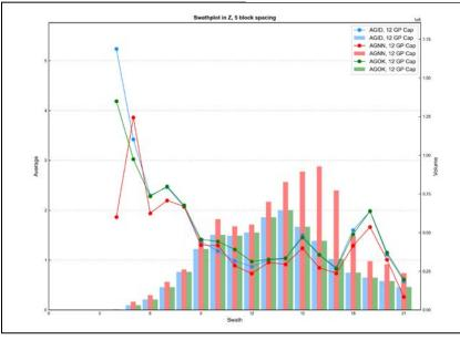
Figure E - 27 Swath Plot in the Z Direction of Silver for the Granite Porphyry
