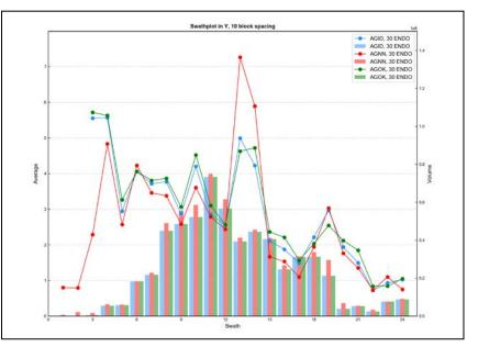
Figure E - 50 Swath Plot in the Y Direction of Silver for the Garnet Skarn
