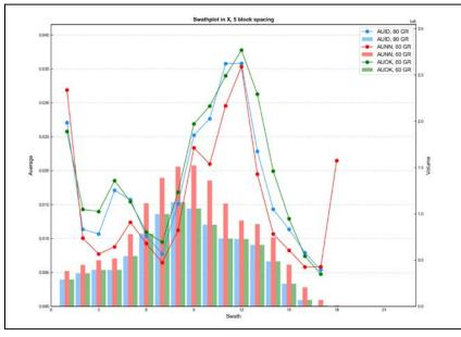
Figure E - 100 Swath Plot in the X Direction of Gold for the Granite
