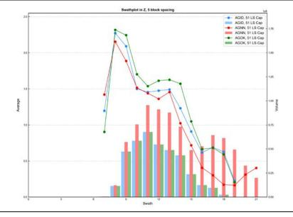
Figure E - 87 Swath Plot in the Z Direction of Silver for the Limestone
