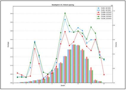
Figure E - 67 Swath Plot in the X Direction of Total Copper for the Pyroxene Skarn
