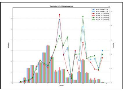
Figure E - 64 Swath Plot in the Y Direction of Gold for the Pyroxene Skarn
