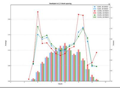
Figure E - 57 Swath Plot in the Z Direction of Total Copper for the Garnet Skarn
