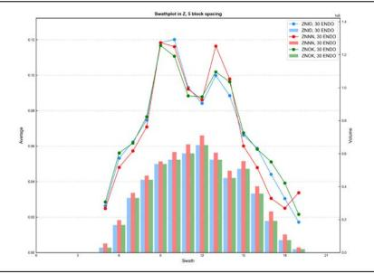
Figure E - 60 Swath Plot in the Z Direction of Total Zinc for the Garnet Skarn
