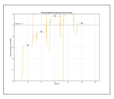
Figure D - 167 Downhole Variogram for Total Zinc in Limestone
