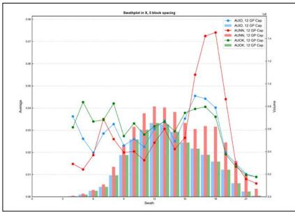
Figure E - 28 Swath Plot in the X Direction of Gold for the Granite Porphyry
