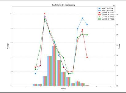
Figure E - 39 Swath Plot in the Z Direction of Silver for the Iron Oxide Breccia
