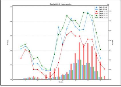
Figure E - 94 Swath Plot in the X Direction of Total Zinc for the Limestone
