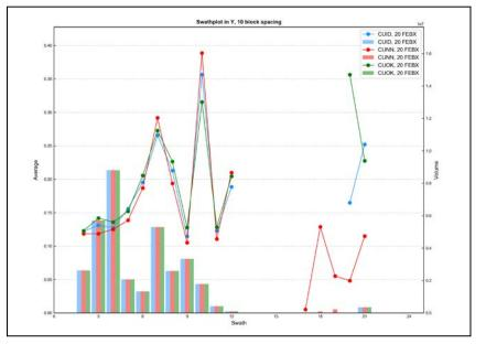
Figure E - 44 Swath Plot in the Y Direction of Total Copper for the Iron Oxide Breccia
