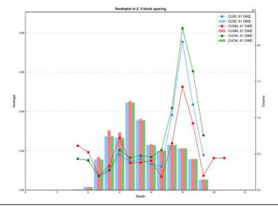
Figure E - 117 Swath Plot in the Z Direction of Total Copper for the Dikes
