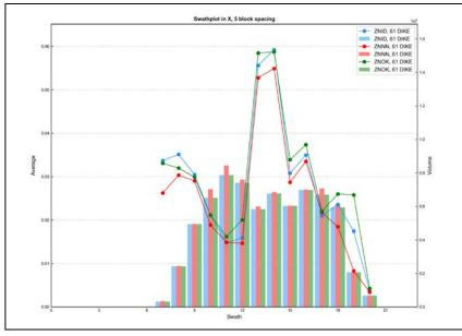
Figure E - 118 Swath Plot in the X Direction of Total Zinc for the Dikes
