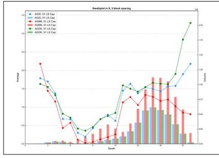
Figure E - 85 Swath Plot in the X Direction of Silver for the Limestone
