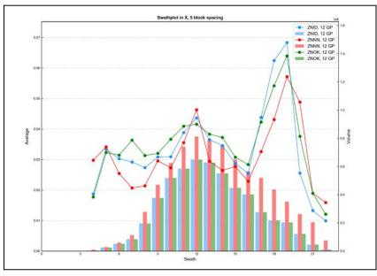
Figure E - 34 Swath Plot in the X Direction of Total Zinc for the Granite Porphyry
