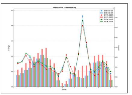
Figure E - 107 Swath Plot in the Y Direction of Total Zinc for the Granite
