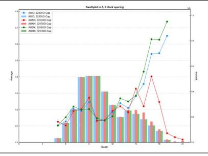
Figure E - 65 Swath Plot in the Z Direction of Gold for the Pyroxene Skarn
