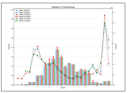
Figure E - 59 Swath Plot in the Y Direction of Total Zinc for the Garnet Skarn
