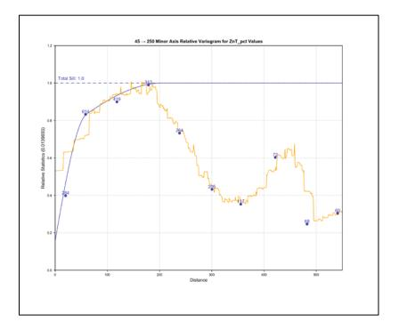
Figure D - 170 Minor Axis Variogram for Total Zinc in Limestone
