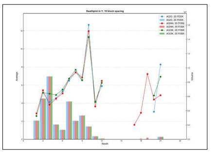
Figure E - 38 Swath Plot in the Y Direction of Silver for the Iron Oxide Breccia
